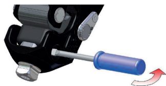
Fig. 20 Removing the Stance-Flexion Rubber
