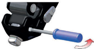
Fig. 20 Removing the Stance-Flexion Rubber
