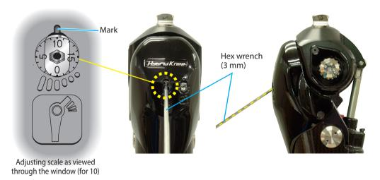
Fig. 11 How to Adjust Hydraulic Resistance
