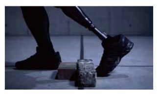
The microprocessor knee is programmed to perceive constant knee position in order to respond to abnormal situations. For instance, if prosthetic side gets stuck on an obstacle during swing phase, the knee can detect abnormal conditions and immediately increase resistance to prevent knee buckling.
