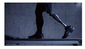
Microprocessor controls hydraulic cylinder and provides a smooth swing phase at various walking speeds. Finely tuned response coupled with the four bar linkage allows for a natural gait. The User will feel how the ALLUX can smoothly transition from stance phase to swing phase. ALLUX four bar linkage is designed for ease of flex at initial swing.
